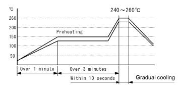
For soldering, please refer to the soldering curves.
