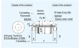
\* Parts are joined by means of silver brazing. (Excluding welding sections)
