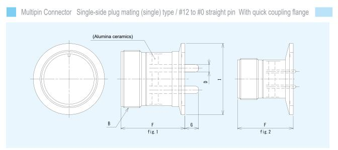
Part materials: Alumina ceramics, Fe-Ni, SUS304, etc. Joining method: Silver brazing and TIG welding
