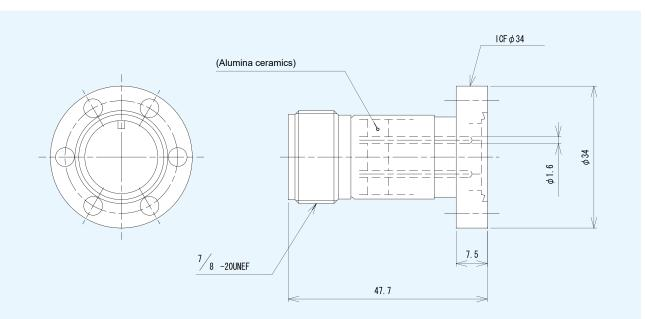
Multipin Connector Single-side plug mating (single) type / #16 straight pins, thermocouple With Ø34 ConFlat flange
