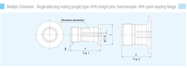
Part materials: Alumina ceramics, Fe-Ni, SUS304, etc. Joining method: Silver brazing and TIG welding
