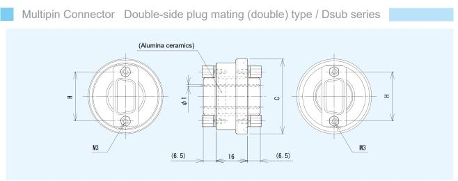
Part materials: Alumina ceramics, Fe-Ni, SUS304, etc. Joining method: Silver brazing and TIG welding
